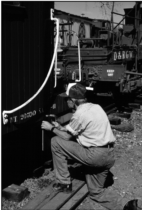
Ralph Vance fits a new piece of siding to fill the gap on the caboose. – Photo © Steve Mason
